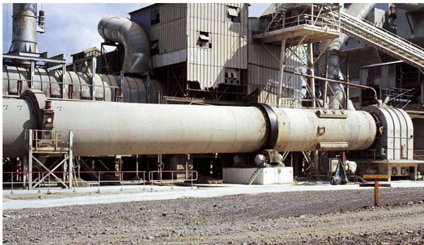
Figure 7: Cylindrical rotary kiln used to make cement 3
