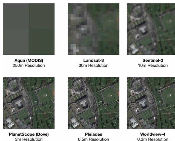
Figure 12 - A visual representation of different satellite resolutions on photo clarity (IPTSAT, 2024)
